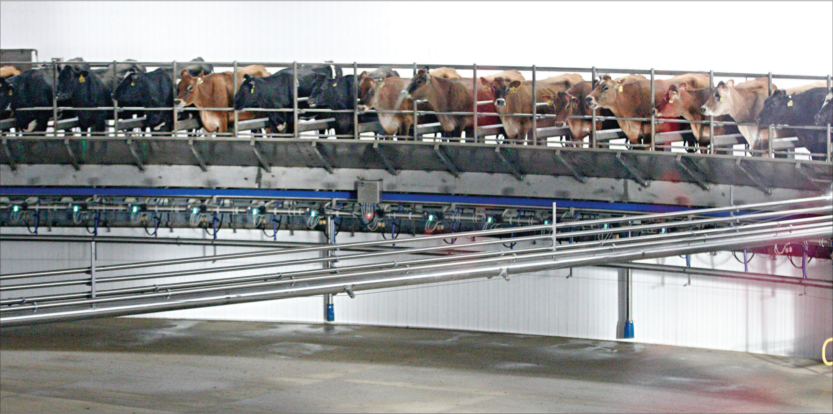
The rotating milking carousel at Clark Dairy can milk 128 cows at one time. The interior carousel is quite a sight to behold.
