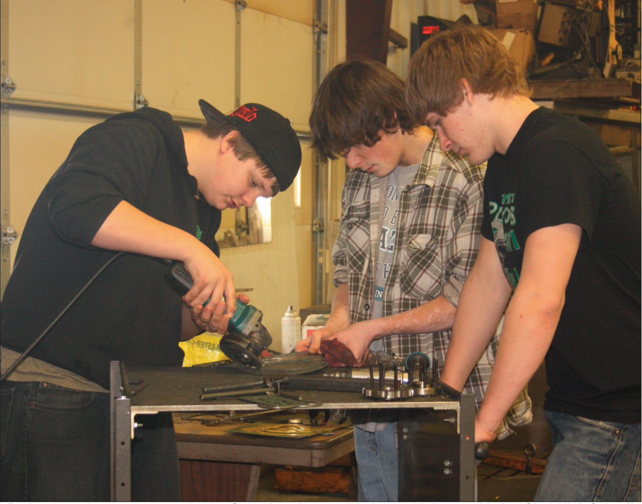
Project-based geometry students Cory Lowrie, Blaze Fischer and Brady Atherton work on smoothing out the rough edges of a project that just came off the plasma cutting table. This table and the computer-aided design (CAD) computers that operate it are new
