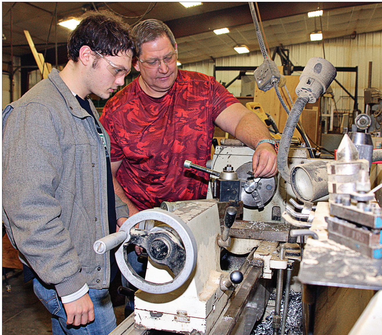
Matt Streff, a sophomore at Clark High School is working on an engine lathe machine that cuts metal by turning, under the guidance of his instructor Todd Jenkins. Learning skills used in the real world while still in high school - Career and Technical Education,
